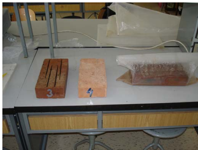
Fig. 1: Wet brick No 3 with channels, dry brick No 4 and brick No 2 wetted in closed carry bag
