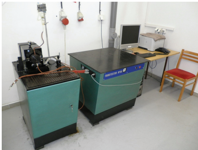
Obrázok 1 Meracie zariadenie Tribotestor M 06 Figure 1 Measuring device Tribotestor M 06
