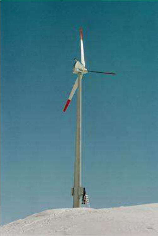
Figure 7 : SmallWindTurbine (SWT), Aventa AV-7
