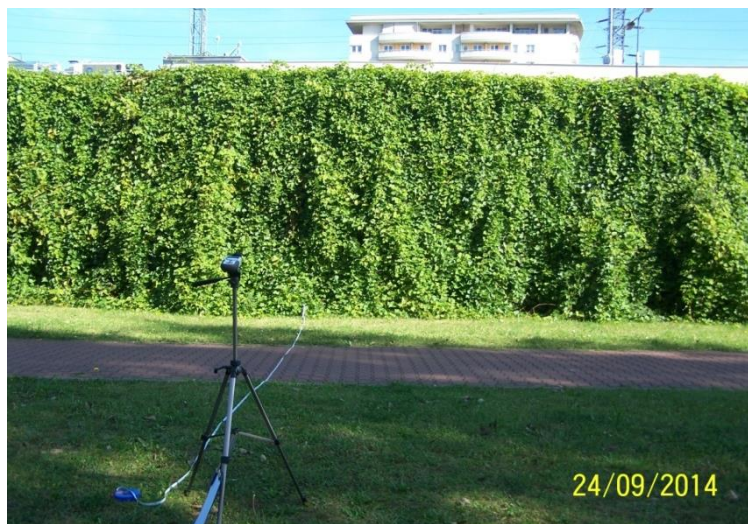
Photo1 The measurement of noise intensity in 10 meters distance from the acoustic screen at Aleja Prymasa 1000-lecia (Draps 2014)
