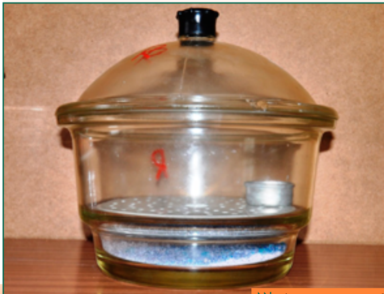
▶▶ The constant weight of the sample is checked after cooling in the desiccator and after re-drying by further weighing
