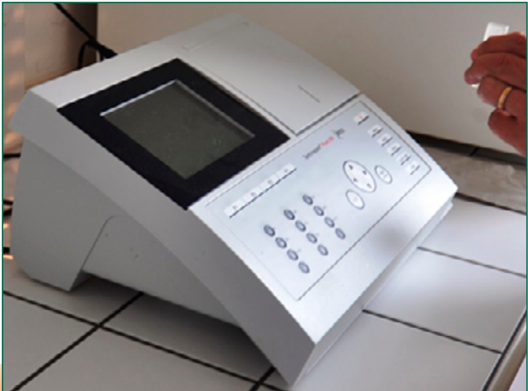
▶▶ The solution of pure petroleum ether is used for setting of calibration zero (BLANK ZERO)
