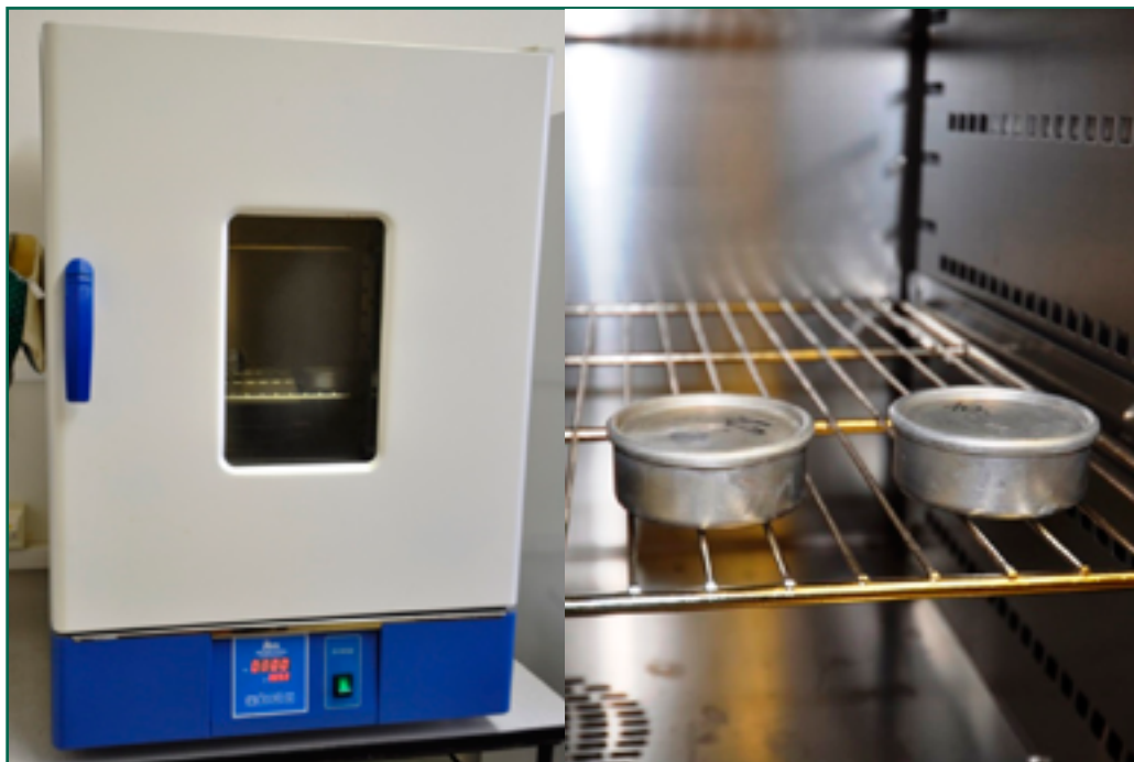
▶▶ The aluminium desiccator with lid and fresh pea seeds is dried at 105 °C to constant weight (approximately 24 hours)
