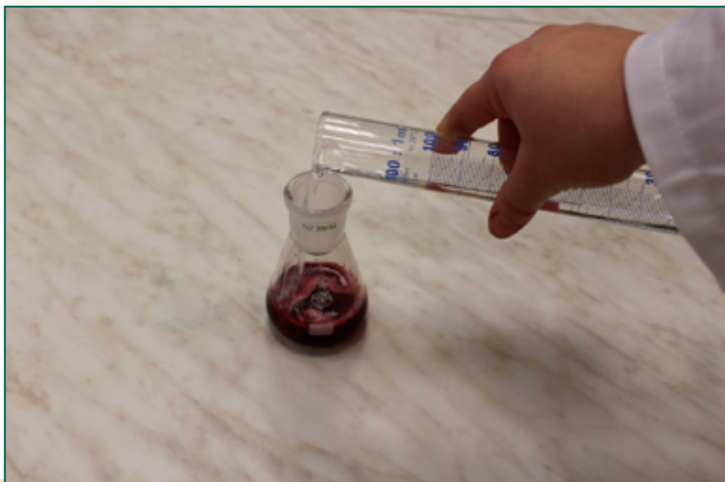
▶▶ The sample is mixed with 40 cm 3 of 70% water solution of ethanol or methanol
