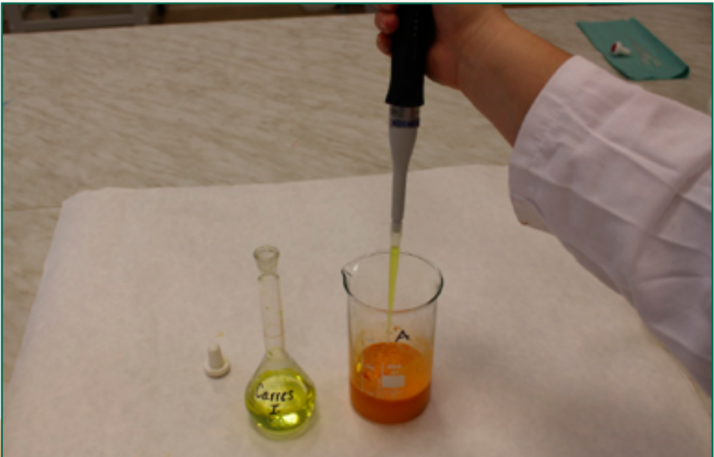
▶▶ Carres I solution (1 ml) is added to the homogenized sample for clarification and the sample is mixed gently
