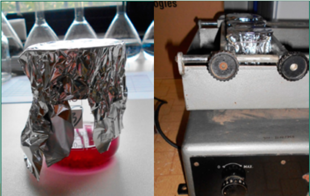
▶▶ The beaker is covered by aluminium foil and anthocyanins extraction to the ethanol is realised by shaking at laboratory shaker (100 revolutions per minute) within 12 hours
