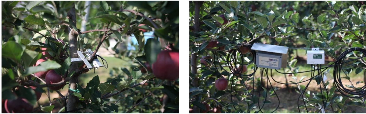
Figure 1 Dendrometer DD-S and datalogger (Kišš, 2018)
