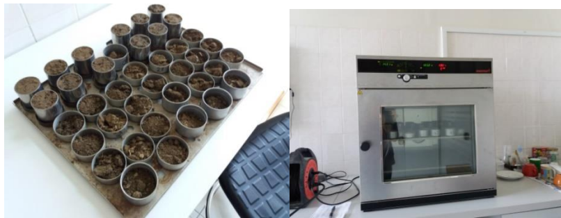
Figure 1 Drying undisturbed soil samples (left) in the oven at 105 °C (right). Disturbed soil samples in the image left were not related to this study
