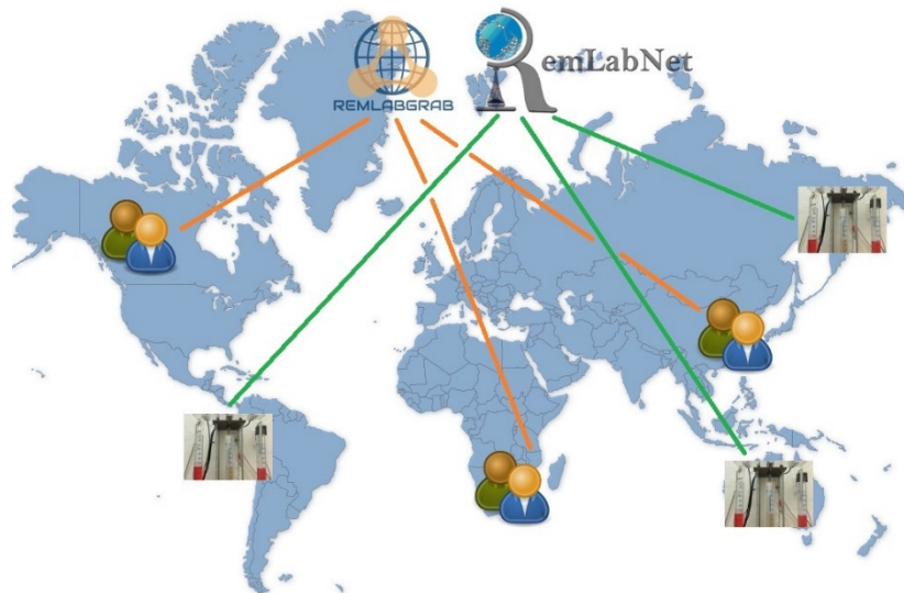
Figure 6 - REMLABNET and REMLABGRAB: Possible connections in our system of RLs: clients via REMLABNET for the measurements on RLs (green line) and supervising personnel via REMLABGRAB to inspect measurements and control data (orange line)
