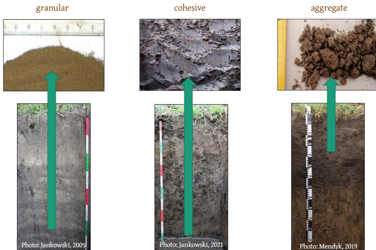
Figure 5.6: Basic types of soil structure A) granular, B) cohesive, C) aggregate (Šimanský, 2022)
