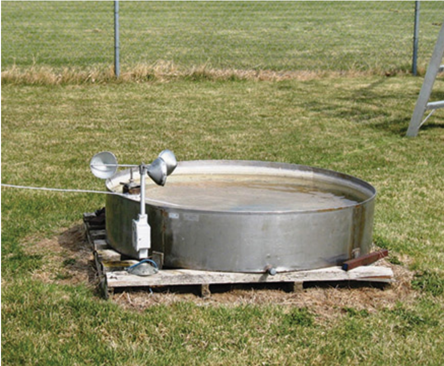
Picture 63 Class A evaporation pan is simple tool to estimate water balance of an environment (extension.okstate.edu)
