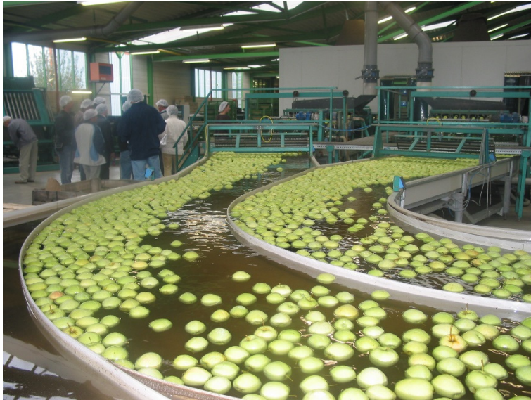
Picture 82 Sorting machine for juicy fruits uses water for fruit conveying (Paulen)
