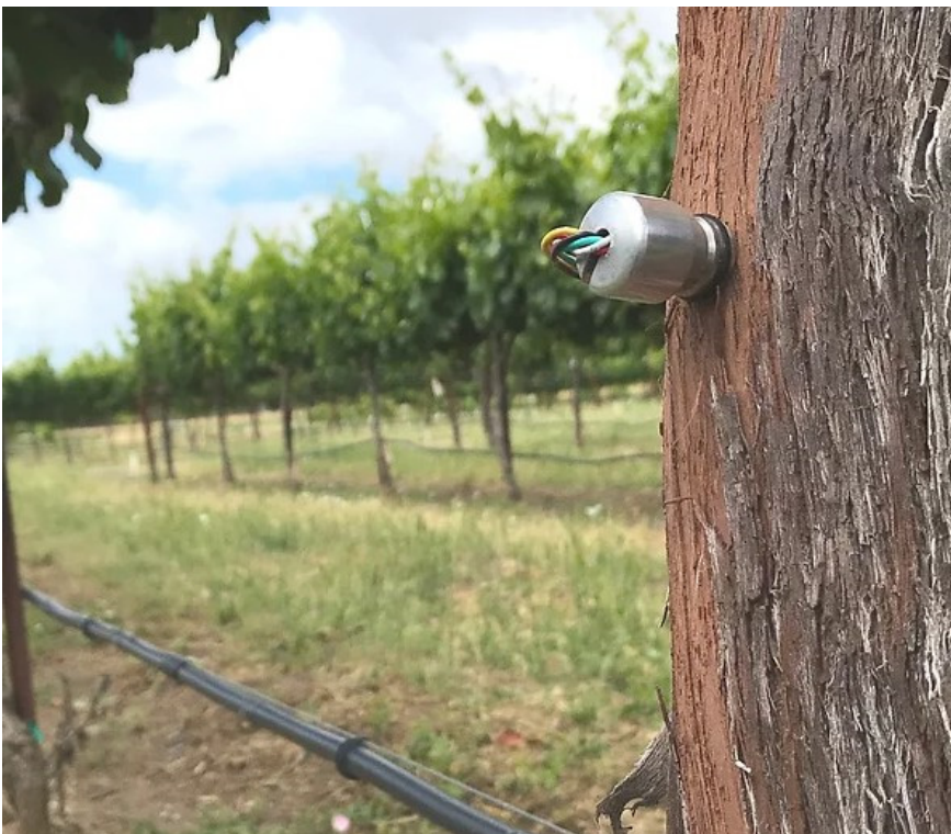
Picture 64 Measuring stem water potential allows to estimate water stress in plant (florapulse.com)
