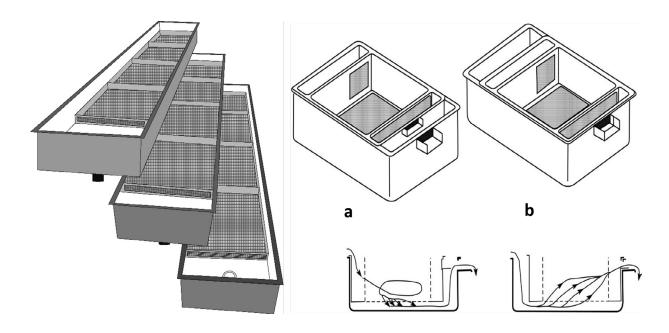
**Picture 5.1:** Clark-Williamson flumes with the incubation liners (1), Rückel-Vack incubation device (2) (Kostomarov, 1958 – edited). a – circular flow, b – bottom flow
