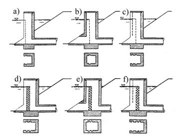
Figure 1.3: Types of outlets (Čistý, 2005): a) open, simple, b) closed, simple, c) open, duple, d) open, simple double, e) closed duple double f) open duple double
