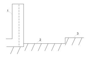
**Figure 1.6:** Fishing pit (Andreji, 1996 – edited): 1 – outlet facility, 2 – fishing pit, 3 – main drainage ditch
