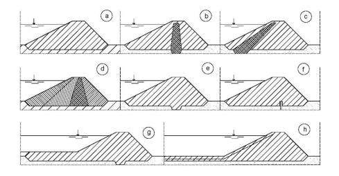
**Figure 1.2:** Types of ground dams (Čistý, 2005): a) simple homogenous dam, b) dam with an internal sealing core, c) dam with a sealing stop, d) heterogeneous dam, e) homogeneous dam with a sealing lock, f) homogeneous dam with a sealing stilt wall, g) homogeneous dam with sealing carpeting, h) homogeneous dam with a sealing membrane from PVC
