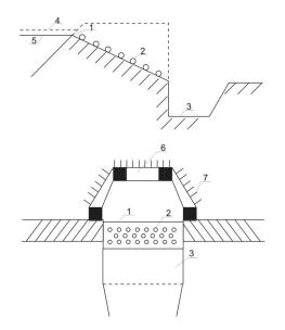
**Figure 1.4:** Front safety overflow (Andreji, 1996 – edited): 1 – overflowing level, 2 – slide, 3 – under-dam pit, 4 – maximum level, 5 – normal, 6 – service bench, 7 – bar screen
