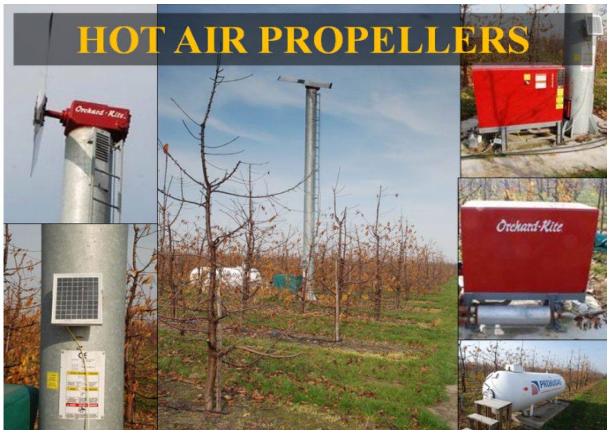
Fig. 12. Stationary propellers are used to mix the air within the orchard. The fog generator creates a layer above the crowns, through which warm air does not penetrate into the higher layers of the atmosphere. It is also used in combination with paraffin candles. (photo: Mezey)
