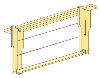
Figure 25 Wooden wired bee frame
