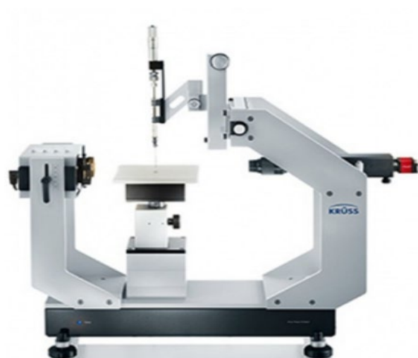
Figure 2 Drop Shape Analyzer - DSA30, manufactured by KRÜSS - a device designed for contact angle and surface tension measurement
